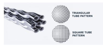
The "twisted" baffle-free arrangement of the tubes provides gaps that facilitate convenient cleaning on the shell side while the round ends of the tubes allow for the use of conventional tube-to-tubesheet joints. Both the profile of the individual tubes and the width of the connection points between tubes can be varied to elongate cleaning lanes, further accommodating routine maintenance.
