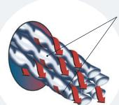
UNIFORM SHELL SIDE VELOCITY CAN REDUCE FOULING CAUSED BY DEAD SPOTS.
